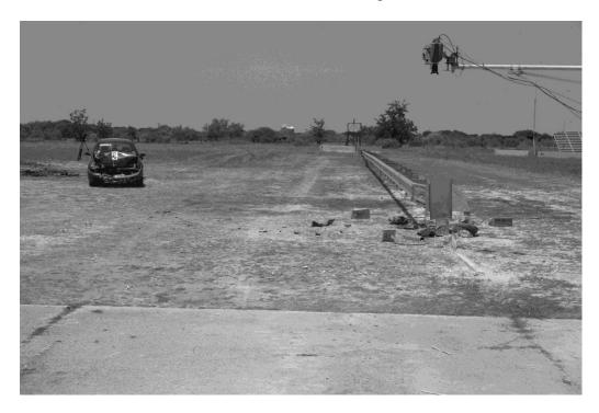
29. Photograph TAMUS007835 contains an angle iron, which is slightly above the ground (especially near support post 1, in the lower left hand corner of the photo). See the enlarged photo below:
