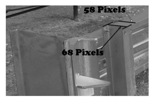
23. Based on the 5.875 inch measurement of the I-Beam, the Rail Feeder Chute is seen to be approximately (58/68) \* 5.875 = 5.01 inches.
