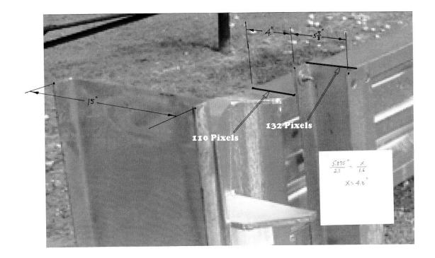
13. I also printed out TRINITY012683, and took measurements of the printed drawing. Using a caliper to obtain precise measurements, and measuring at the center of the I-Beam, I found the I-Beam to be approximately 1.26 inches wide, while the Rail Feeder Chute was 1.04 inches wide. Based on the 5.875 inch measurement of the I-Beam, the Rail Feeder Chute is seen to be approximately (1.04/1.26) \* 5.875 = 4.85 inches wide.
