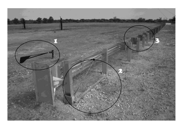
25. Photograph TAMUS007835 contains a stake and guide cables to guide the Pickup Truck into the guard rail at the proper point. This is shown enlarged below:
