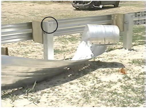
35. Therefore, in my opinion, TAMUS007835 is a photograph of the Truck Test, a test of Pickup Truck Redirection at beginning of length of need (3.8 m (12.5 ft) from terminal beginning). It is not a photograph of the Small Car Test at end-on, at quarter-point offset.
