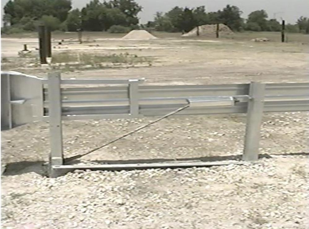
31. In the Small Car Test, the angle iron is buried in the ground to a much greater extent. See, for example, the following screen capture from 2:19 and 2:28 of the video, respectively. As can be seen, there is no slightly-above-ground angle iron; instead, the angle iron appears to be fully buried in the ground.
