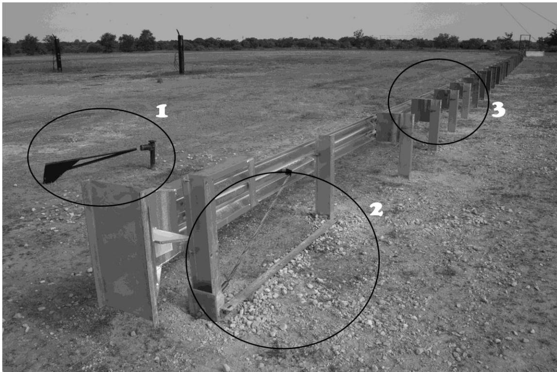
25. Photograph TAMUS007835 contains a stake and guide cables to guide the Pickup Truck into the guard rail at the proper point. This is shown enlarged below:
