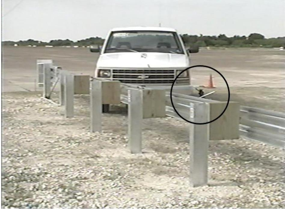
27. This stake and guide cables set up in a completely different manner in the Small Car Test, since it is an axial test. See the following three screen captures from 1:42, 5:14 and 5:35 of the video, respectively. In all three cases, the stake and cable are clearly absent from the location as shown in TAMU007835
