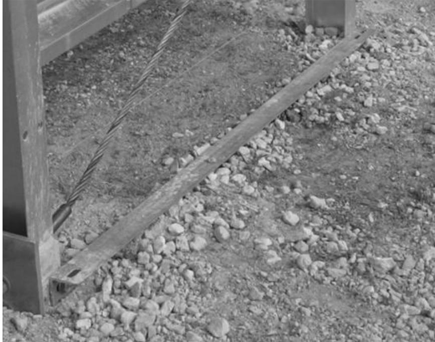
30. This slightly-above-ground angle iron is present in the Pickup Truck Test. See the following screen capture from 7:03 of the Pickup Truck Test video. In this case, the slightly-above-ground angle iron (near the first support post) can be clearly seen.
